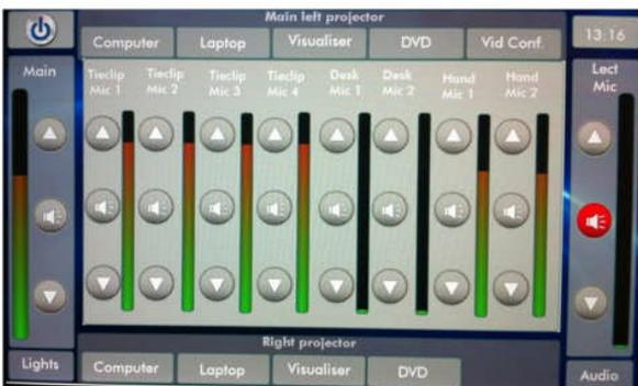
**To use the lectern mic.** Turn it on at the AMX by pressing the lectern Mic light (red for off, white for on). Set the volume at about 50% although this can go up or down depending on the height of the speaker. Don't use a tie clip at the same time or feedback will occur.
