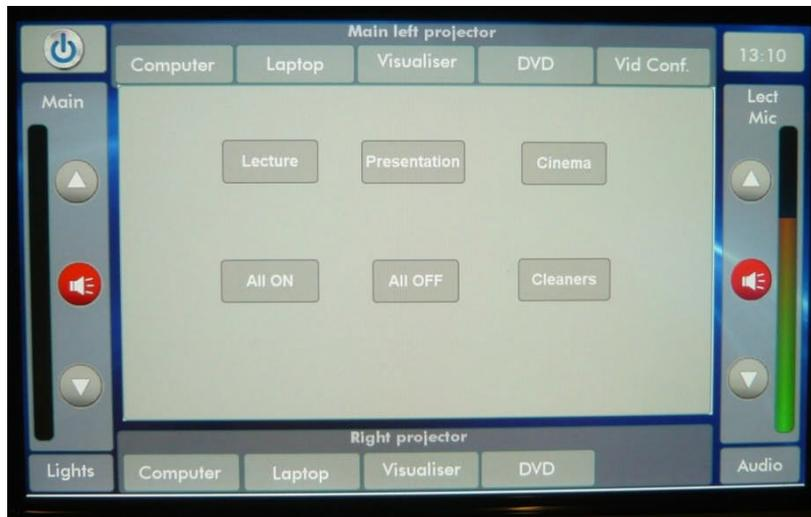
Note that when the 'lighting button is pressed then the other functions are not available until the lighting panel turn off after about 15 seconds.
