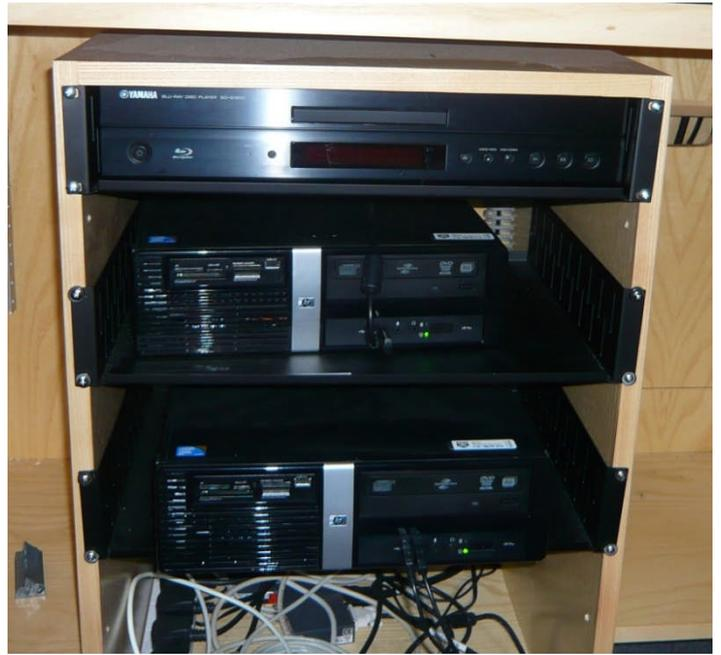
The left hand keyboard and mouse controls the main (left) PC and the right hand keyboard and mouse controls the right PC. The Sympodium screen is the confidence monitor of the left (Main) and the vertical monitor is the confidence monitor for the right PC. These should not be switched round.
